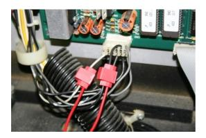
With the aid of two cable clamps connect the included power cable to the black and grey/white wires.
