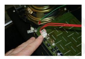
Connect the display power supply to the display.
