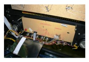
Remove the three mounting screws and remove the metal cover plate.
