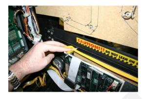
Cut the cable tie of the grounding wire.
