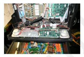
Reinstall the display driver board and fix it with the four Philips screws. Reconnect the flat cable and the power supply cable. The original power supply connector is not in use any longer. Store it in the back panel and fix it to the cable harness with a cable tie.
