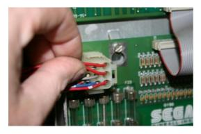
Connect the included display power supply cable with the two red wires at J17 pin 1 and 4.
