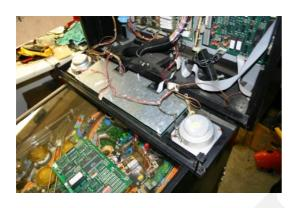
Remove the four mounting screws of the display driver board and remove it.
