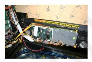
Remount the metal cover plate. Reinstall the three spacers and reinstall the display driver board. Fix the grounding wire with cable ties.
