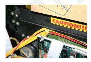
Use cable ties to fix the grounding wire and display power supply cable.
