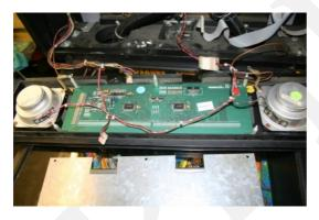
Remove the four spacers of the display driver board, both nuts and remove the metal cover plate.
