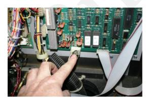
You will find the unregulated 12VDC at connector CN2 on the soundboard.
