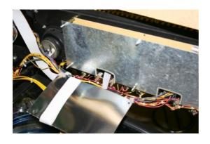
Remove the four mounting screws of the display driver board and remove it. Remove the three spacers too.
