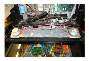
Put the metal cover plate back on and fix it with the two screws and the four spacers.
