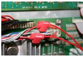
Use the two include cable clamps to make the connection at J17 pin 1 (red) and 4 (red).
