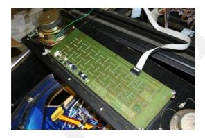
Fix the new display and reconnect the flat cable.
