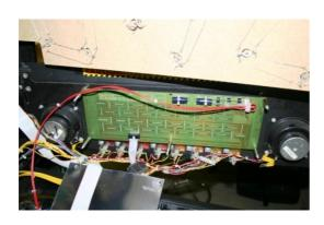
Reconnect the flat cable and the included display power cable. Fix the washers and spacers back on.
