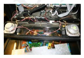
Remove the five mounting screws of the old display and remove it.
