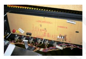
Remove both cable connections. Remove the spacers and washers from the five long mounting bolts.
