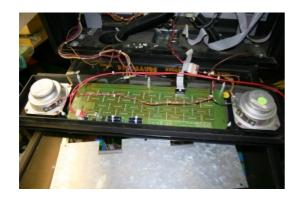
Install the new PinLED display and remount the five mounting screws. Connect the flat cable and the included display power cable.
