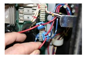
With the aid of two cable clamps connect the included power cable to 9VAC at the red cables, which reach the board at J101 pin 1 and 2
