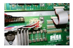
Slew the speaker panel aside. J17 on the I/O power driver board. You have to connect the included display power cable later here.
